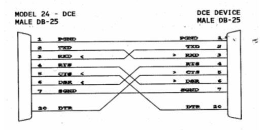
Figure 6-Model 24SII (DCE) to DCE Device
